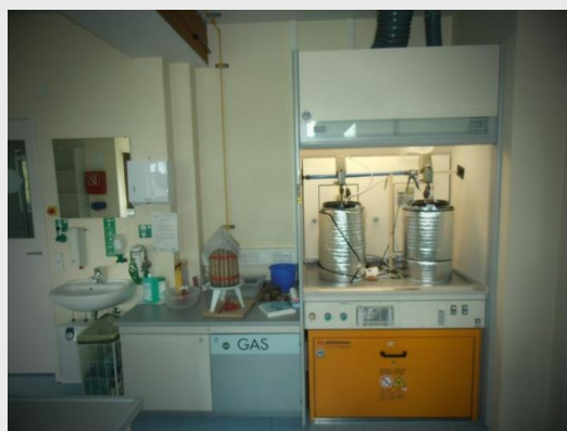
Lab-scale batch digesters and de-watering station
